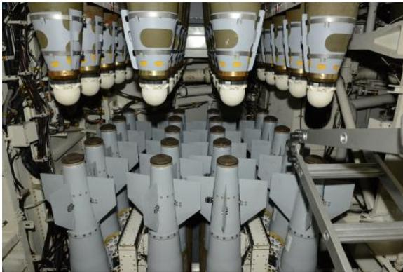
The B-2 can carry 80 of these 500-pound bombs, each guided to detonation with GPS coordinates. Each of the bombs can be programmed to hit a specific target, at a specific altitude, from a specific angle, at a specific time. "These were pretty tight shot groups, and the B-2s could attack them on a single pass," Vander Hamm says.
