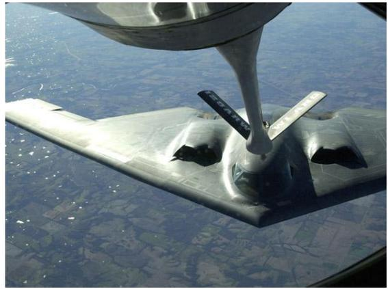
The B-2's fuel port is on top of the fuselage, so a pilot can't tell how close the boom is to the bomber's receptacle. They watch lights under the tanker plane's fuselage that tell him to move forward, left, or right. Once the connection is made, a dashboard screen says "LATCH" and the fueling begins. As thousands of gallons of flow, the B-2s flight control computer routes it to the appropriate tanks as a way to preserve the bomber's center of gravity.
